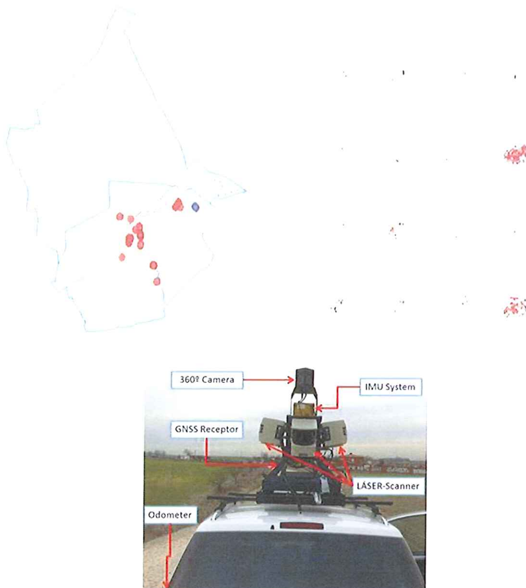
Fig. 2 Map municipality of Alcorcon (INGRID System) and detail of IPS2 (Mobile Mapping System)
