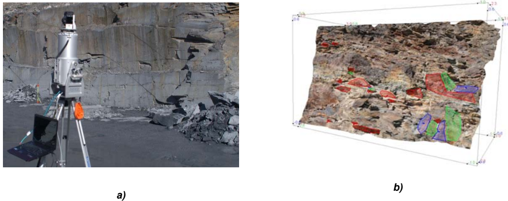
Fig. 3 Measurements in the slate quarry using the RIEGL® LMS-Z390i scanner a) and points cloud obtained by laser scanning with the joint sets b).
